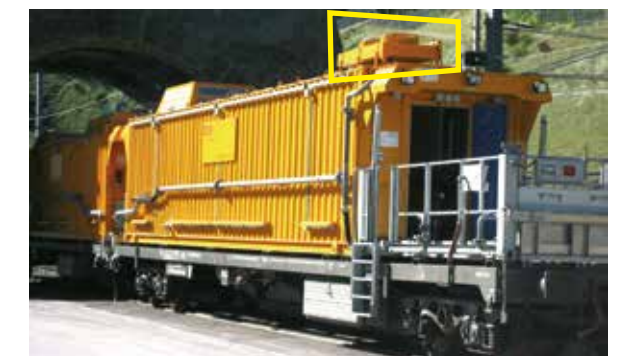
Radiator mounted separately on wagon roof
