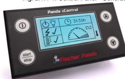
Fig. 2.1.1-1: Control Panel - Generator
